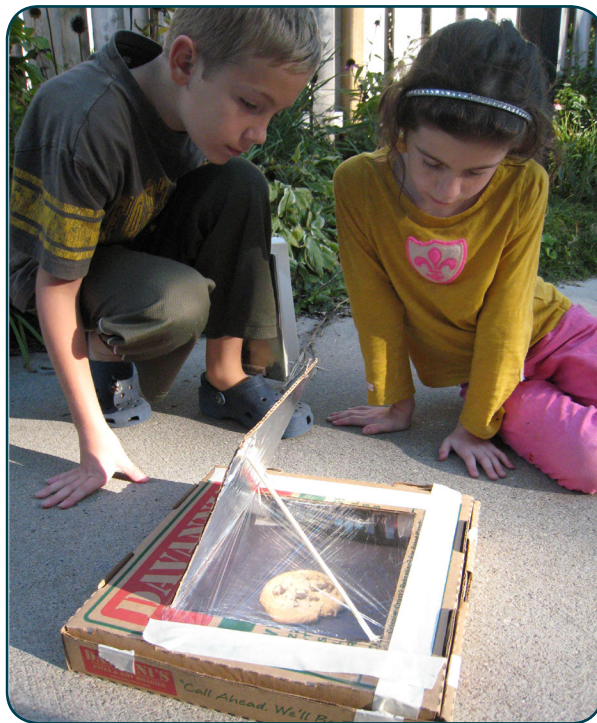
(An example of a simple solar oven made with a pizza box and some foil. Photo: Liz Heinecke, NASA Earth Ambassador)
